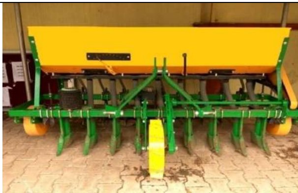
Fig.1. Stationary view of tractor operated FYM manure applicator with agitator unit
